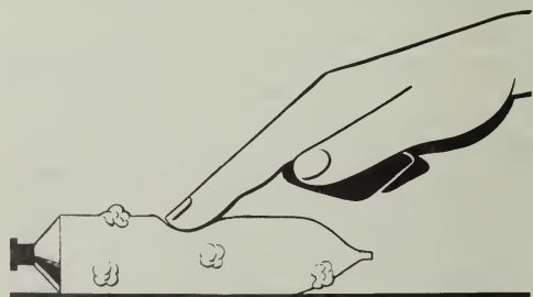
Figure 10-5.—Pressure is transmitted in all directions.
